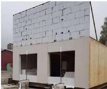
Photo of the compartment at the end of assembly, before starting the test
