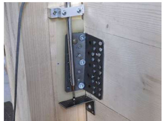
Monotonic shear test ( F_{2/3} ) on NINO15080 in timber-to-timber configuration.
